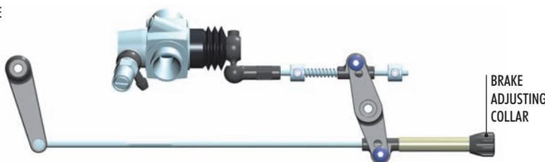
Adjust the composite collar on the brake linkage so the brakes work smoothly.
