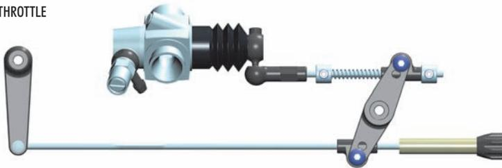
With the engine NOT RUNNING but the receiver turned ON, apply full throttle at the transmitter.
