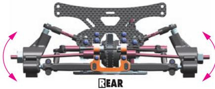
When the bars are set, verify that both sides move at the same time. If they do, the bars are set up correctly. If not, make sure that both downstops are the same and that the bar wire is flat.
